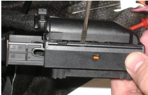
FIGURE 1 REMOVING TOP COVER
